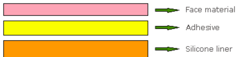
Fig. 2: Structure of the self-adhesive product.
